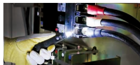
Maximum sensitivity variable range 40 V to 80 V.A.
